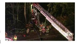
against another tree and would not provide access to the driver. The passenger side door would have been too much of a drop off to access the driver and would have put the crew on the downhill side of the vehicle. Engine 45 utilized Kent's Ladder 74 to attach Engine 45's winch cable to the vehicle and secure car from tipping over. Engine 45 cut the windshield out of the vehicle and extricated the driver with the attic ladder. The driver was not injured and required no medical attention.
