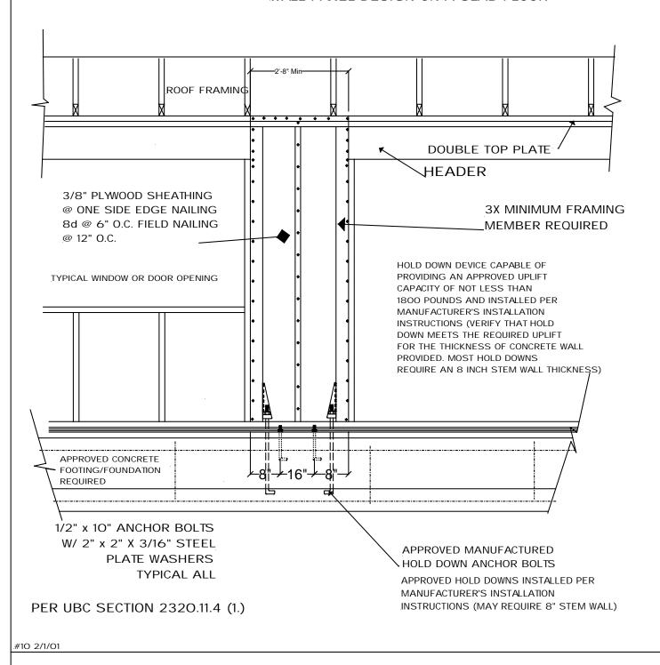
1 STORY 2'-8" SLAB ON GRADE ALTERNATE BRACED WALL PANEL
