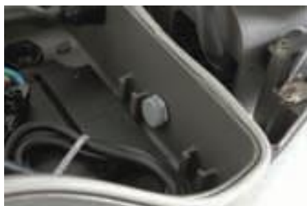
+ IP 68 vent prevents condensation and regulates pressure and temperature variations
