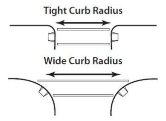
The longer the radius of a curve, the faster a vehicle can move around that curve – as many pedestrian witness when, in crossing at an intersection, they are confronted by a car whizzing around the corner seemingly out of nowhere. Reducing a corner radius to somewhere between one and twenty feet can:
