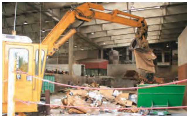
A Transfer Station Operator recovers cardboard from a mixed load of solid waste
