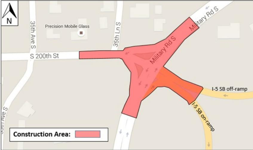
Construction work by WSDOT is continuing on the Southbound I-5 interchange at Military Road South and South 200th Street. This work will widen and realign the intersection and install new traffic signals to allow for easier access between I-5 and, the Angle Lake Light Rail Station, and the City of SeaTac. Please plan alternate routes around the area if possible. Please contact 440.4DOT (4368) for any noise related complaints or the 24-hour construction hotline at 888.298.2395.
