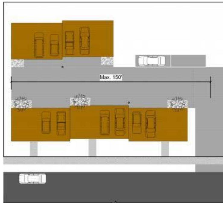
Figure: AUTO COURT MEASUREMENTS Illustration of how the length of an auto court is measured.
