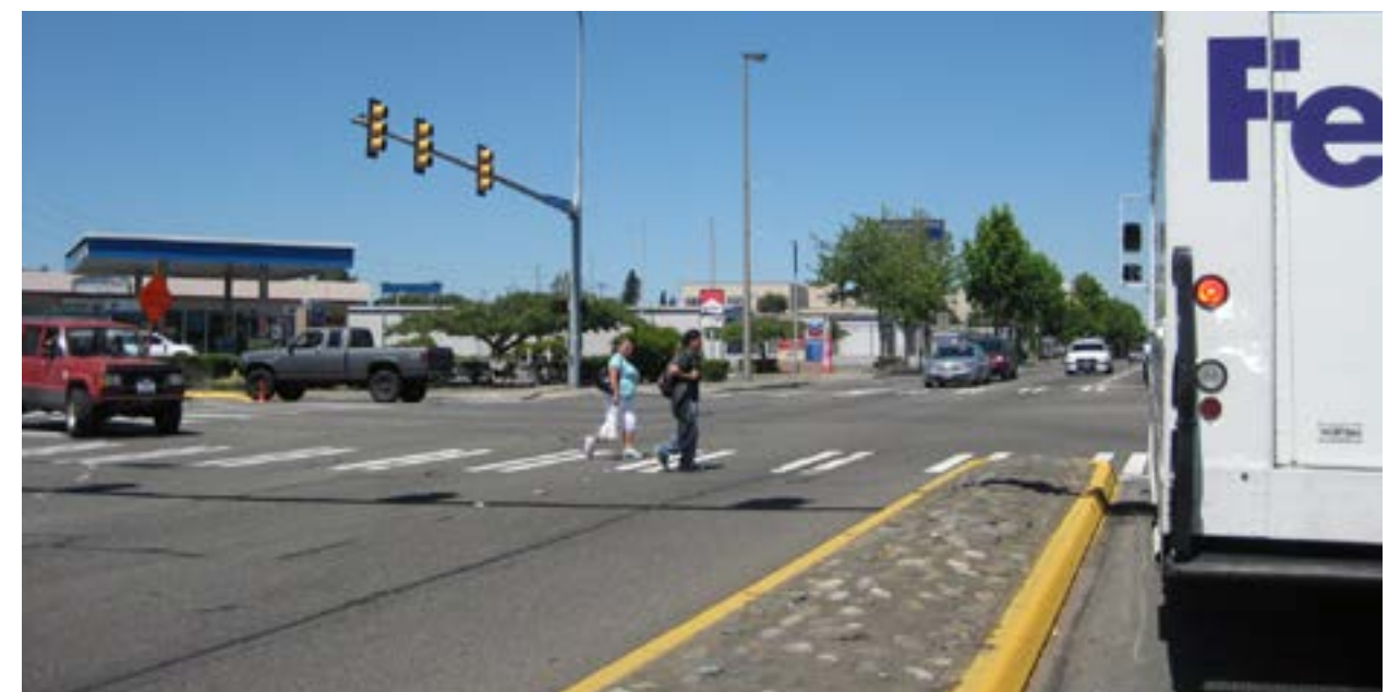
Existing medians along International Boulevard do not provide pedestrian refuge.
