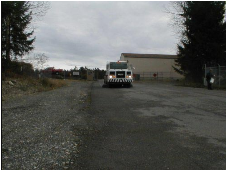
A sweeper picking up debris and soil particles on a paved access road
